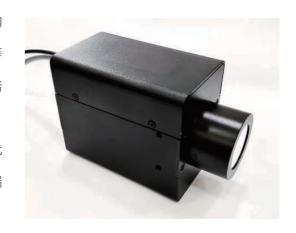
M3013  $\beta$  detector can measure low energy  $\beta$  ray, because of its excellent anti-interference ability, can be widely used in environmental detection, precision measurement, scientific research and other fields. The M3013  $\beta$  detector is mainly composed of end window photomultiplier, high voltage power supply module, signal forming circuit, scintillator and so on.
