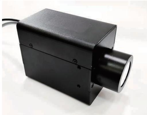
M3012  $\beta$  detector can measure low energy  $\beta$  ray, because of its excellent anti-interference ability, can be widely used in environmental detection, precision measurement, scientific research and other fields. The M3012  $\beta$  detector is mainly composed of end window photomultiplier, high voltage power supply module, signal forming circuit, scintillator and so on.
